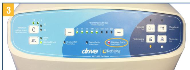
Adjust the weight of the patient using the (+) and (-) button on the weight adjustment scale\*; if the "Low Pressure" LED goes out and the "Normal Pressure" LED is lit, the patient can be placed on the system.
