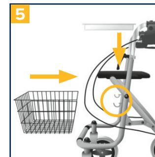
Hook in the basket in the hooks at the frame under the seat plate and place the tray with its small feet in the holes in the seat plate (see picture).
