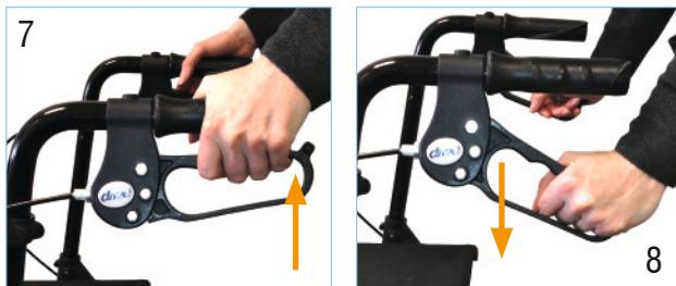
The braking effect of the parking brake acting on the rear wheels can be metered and depends on force applied.
